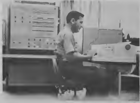
THE SYSTEMS panel lights up like a X-mas tree when in operation. The status of data being processed is indicated on this unit. In the foreground Pedro Yarzagaray enters operating instruction via the printer keyboard.
